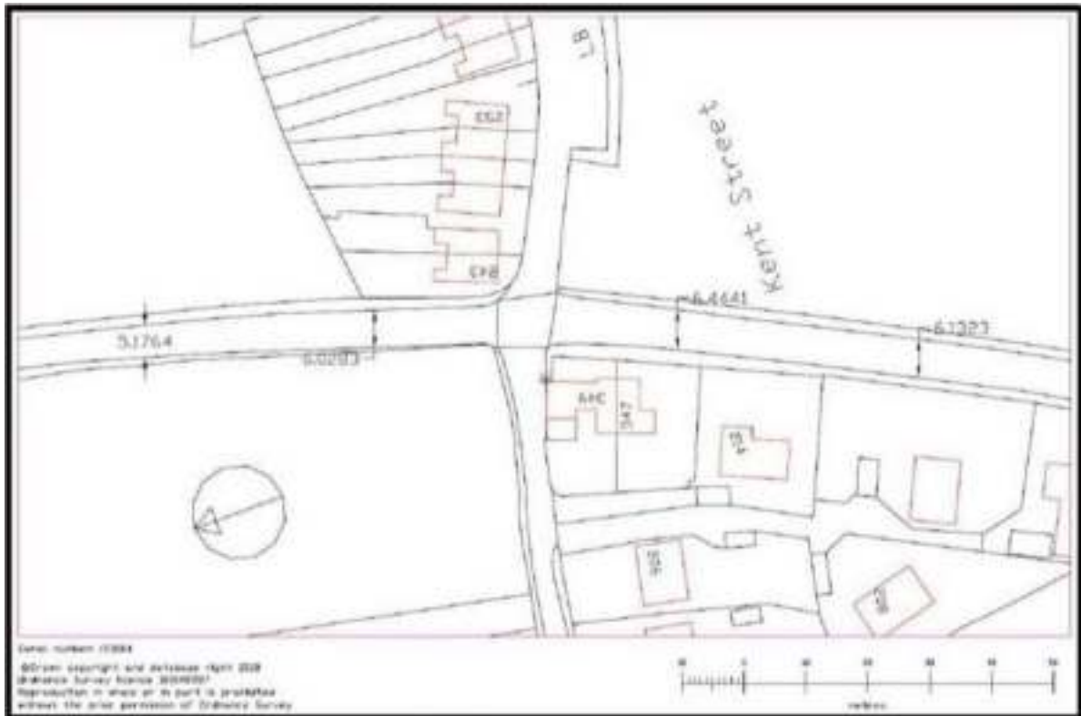
Figure 5: A228 Carriageway Widths
